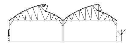
Unique truss design for peak venting: Atrium vent (left) and ridge vent (right). Sidewallls can be vented with an exterior drop-down guillotine (EDDG) vent (left), swingout vent (right), or roll-up sidewall curtains (not shown).
